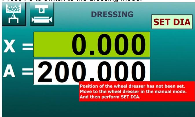
Press the **SET DIA** button for 10 seconds. This will set the new position of the diamond dresser and the calibration has been completed.
