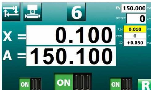
moves to the home position for grinding. Grinding is started with a hand lever. Increments at the reversal points can be switched off while grinding with the left/right bottom buttons.
